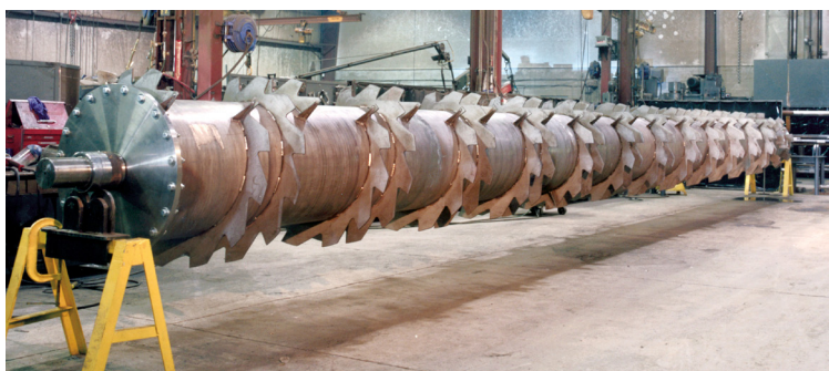
36' long, 38" diameter 2205 duplex SS pulp screw
