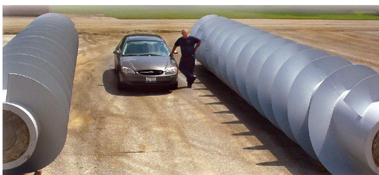
46' long, 78" diameter double lead water lift screws
