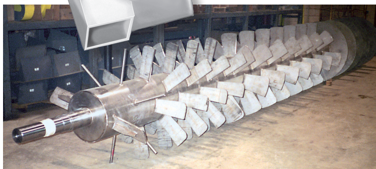
30' long, 48" diameter 316SS paddle type screw
